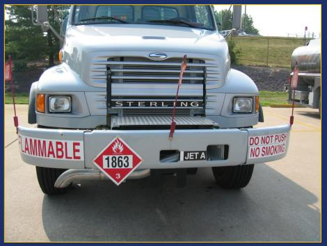
Most fuel trucks have the muffler and exhaust pipe at the front of the vehicle where it will be clear of fuel tanks and piping in the event of a leak.
