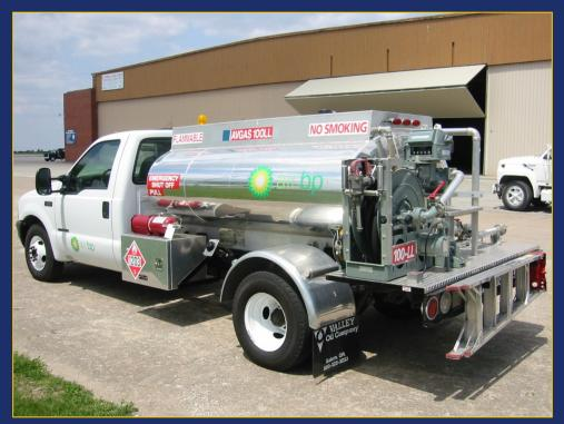
Aircraft fuel servicing tank vehicles are vehicles having a cargo tank used in the transportation and transfer of fuel into or from an aircraft.
