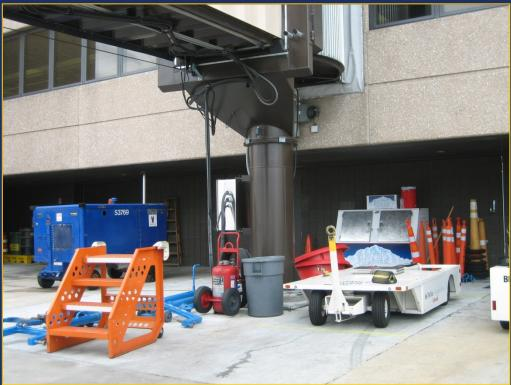
For normal, single parking configurations, extinguishers specified for protection of fuel servicing operations should be located along the fence, at terminal building egress points, or at emergency remote control stations of airport fixed-fuel systems.
