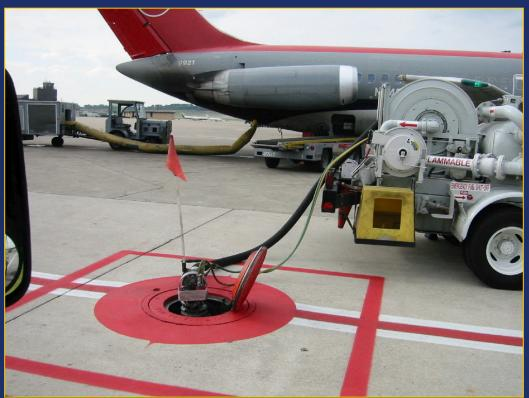
Aircraft fuel servicing hydrant vehicles do not have tanks. These vehicles connect to a pressurized Airport Fueling System hydrant and transfer the fuel to the aircraft through a filter.
