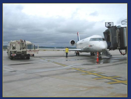
Aircraft fuel servicing vehicles and carts shall be positioned so that a clear path of egress from the aircraft for fuel servicing vehicles shall be maintained.
