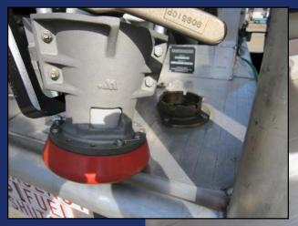
Aircraft fuel servicing vehicles shall incorporate an integral brake interlock system that prevents the vehicle from being moved until all hoses are properly stored.
