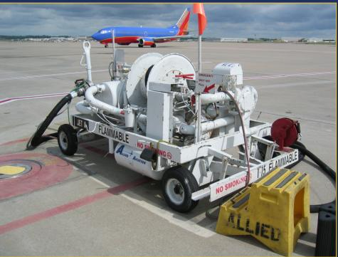
Aircraft fuel servicing carts are equipped with facilities to transfer fuel between a Airport Fueling System hydrant and an aircraft and are normally parked at a fixed location near a gate.
