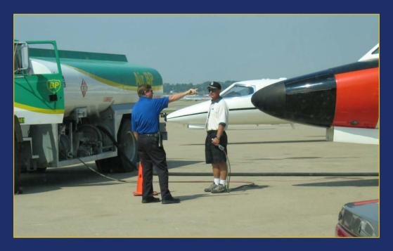
Observe fueling operations while inspecting aircraft fuel servicing vehicles to check for compliance with fire safety standards. In particular, check for proper bonding procedures and use of deadman controls.
