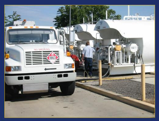
A bonding connection shall be made between the cargo tank and the loading rack before any fuel connections are made and shall remain in place throughout the loading operation.
