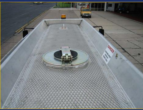
Look for signs of fuel leakage around the dome cover, indicating a problem with the dome cover seal or gasket. Physically inspect the dome cover gasket to check the condition and presence of a gasket.
