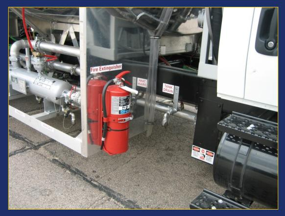
Two fire extinguisher are required on fuel servicing tank vehicles, with one mounted on each side.
