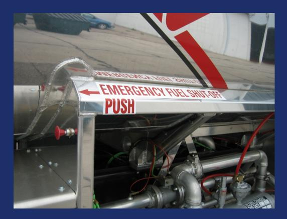
For pneumatic operated emergency shutoffs, fuelers must be started up and placed in pump mode in order to check the emergency shutoff system.
