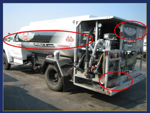
Each aircraft fuel servicing vehicle or cart shall have a sign on each side and the rear to identify the product. The sign shall have letters at least 3 inches (7.62 cm) high and shall be of a color contrasting sharply with the sign background for visibility. The word FLAMMABLE and the name of the product carried, such as JET A, JET B, GASOLINE, or AVGAS shall appear on the sign.
